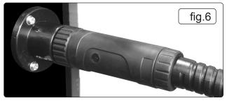
**4.6. CONNECT THE TORCH CABLE TO THE WELDER.** Align the pins on the Euro connector with the socket on the welder front panel as shown in fig.5. Push the connector into the socket and rotate the locking ring (A) clockwise so that it draws the plug into the socket as shown in fig.6.
